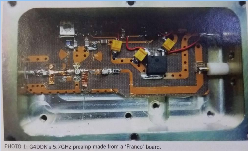
PHOTO 1: G4DDK's 5.7GHz preamp made from a 'Franco' board.
