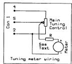
A tuning indicator meter may be fitted if required. It should have a sensitivity of 1mA or greater. A series resistor will be required. The value of which can be calculated by R = 18 divided by the FSD current of meter. Alternatively a 470K pre-set could be used and adjusted for meter FSD. with the main tuning control at max. frequency.
