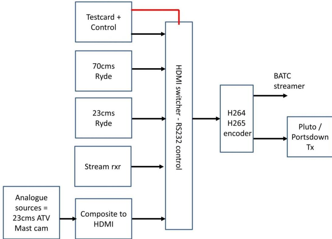
The core of the proposed system is a consumer IR controlled HDMI switch – these are readily available of Multimedia home systems from the normal sources and come in 2 / 4 / 6 / 8 input configurations.
