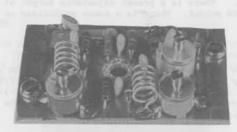
144PA4 - Due to demand for a board of higher specification than the PA3, the 144PA4 was evolved. This has a low loss input circuit to reduce noise figure to under 2dB. The board is larger than the PA3 as it also includes an attenuator after the amp to improve large signal handling. The board measures 2.9" x 1.25" so if you have room then it is to be prefered to the 144PA3.
