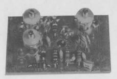
70PA5 - A dual gate GaAs MESFET pre-amp using a 3SK112 or similar device. The noise figure will be typically 1.8dB and gain 16dB. These values could be improved by experienced constructors with minor changes to the board. Our usual input PIN protection circuit and post amplifier attenuator/line feed facilities are fitted as standard. This board is currently the best we offer for 70cms. Board size 2.6" x 1.2"
