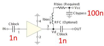
Test Board includes case, connectors, and components (in bold) soldered to PCB
