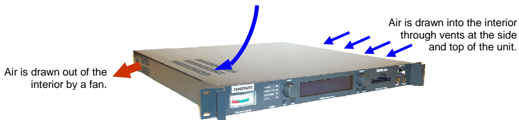
Figure 2.1: Air flow Through the Equipment
