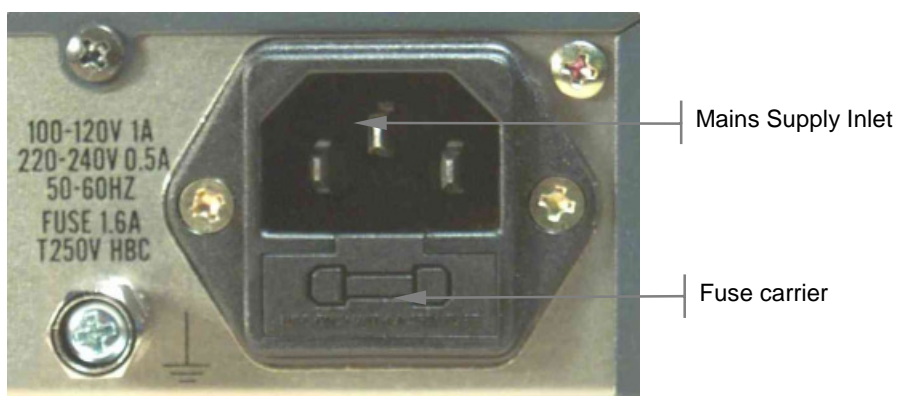
Figure 2.2: AC Power Inlet and Fuse
