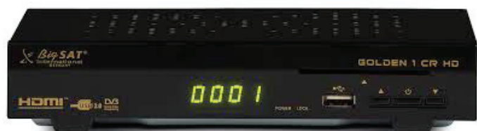
► The popular BigSat set-top-box, used for receiving DATV
