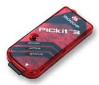
PICKit3 connects to your PC via a supplied USB cable. There will also be a ribbon cable to interface to the programming connector on your oscillator PCB.
