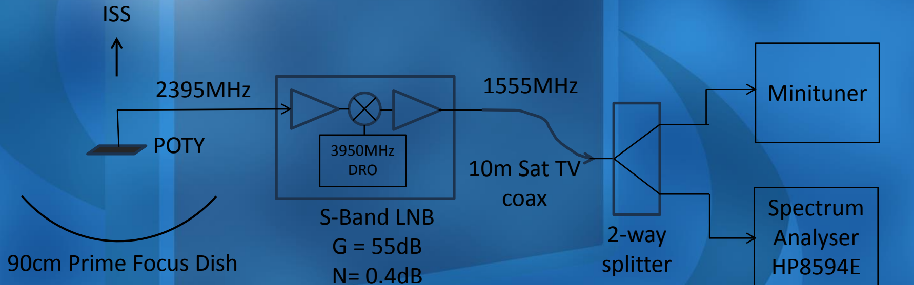
S-Band LNB Test Setup
