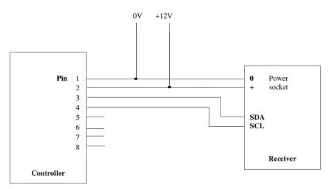
If you want to mount the receiver a long way from the controller, you can use Philips I<sup>2</sup>C Bus Extender ICs type P82B715. You will need one at each end of the control cable. We have used these ICs to control a receiver via more than 50m of cable. P82B715 ICs are available from Farnell and other suppliers.
