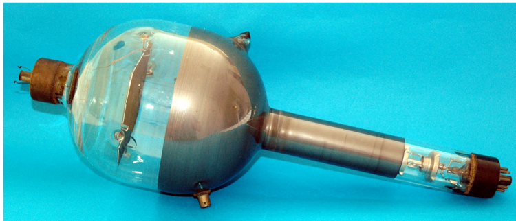
An early shape Monoscope tube by Cathodeon
