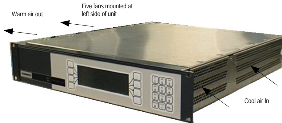
Figure 2.1: Air Path through the Enclosure
