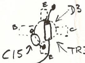
C15 must be as close to TR3 as possible and zero lead length
