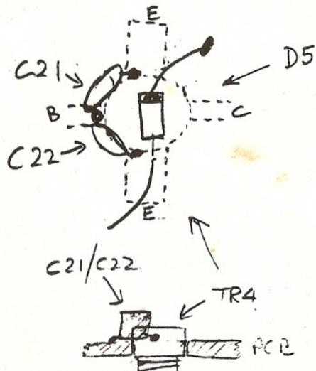
C21/C22 must be as close as possible to transistor body and have zero lead length
